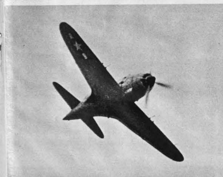
Fast high-powered fighter, Jack has a tail extending aft of tailplane. Fat fuselage resembles no other Jap single-engine type except George.
